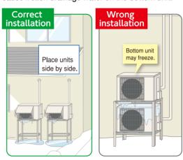
Use a stand with a steel framework that allows water to drain properly. The width of the stand's base must not exceed the width of the unit.
