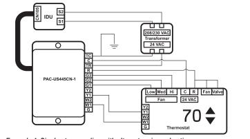
Example 4: Single-stage cooling with alternate primary heating source Note: For this configuration, it is recommended to set SW2-6 to the ON position. Follow the wiring from Example 2 with the following adjustments:
