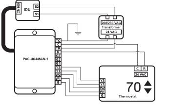
Example 2: Single-stage cooling and heating
